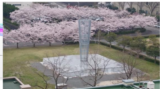
Fig.7. A wind solar tower for field experiment, tower 10m high, collector 15m 2 , at RIAM, Kyushu University
