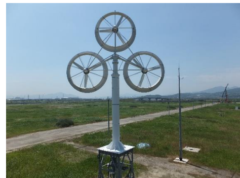
Fig.3. 10kW multi wind-lens turbine using three 3kW wind-lens turbines at Kitakyushu city, 2017 March
